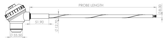
**FLS** – Comes with a full-length ceramic sheath running the entire length of the probe. The ceramic sheath provides a measure of protection to the sensor tip from direct exposure to corrosive and high velocity gases, reducing overall wear. This option provides some protection from particulates associated with wood firing.A 1" BSPT or NPT compression fitting is available for this sheath option.
